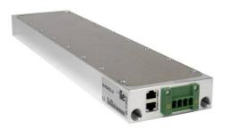
They are designed to drive uv-lamps in a wide range of applications, e.g. label printing (narrow web), container printing, CD/DVD production i.e. in any application which uses uv-lamps up to 8,000 W nominal power.
