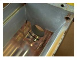
5) Mount the posterior Lamp holder in such a way that the big hole (diameter 17 mm) will be closer to the radiation apertur of the reflector unit (print substrate) so that the lamp can be mounted closer to the print substrate.
