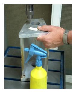
2) Tap the M4-thread from the outside to the inside (use lubricant). Because of the thickness of the end plate a long screw tap is necessary. Please make sure the possibility to use the tap from the inside.
