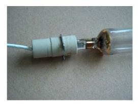
7) Install of the lamp: Thread the lamp-cable through the posterior holder and shift the lamp through the hole of the lamp holder till the circlips get in contact with holder. Put off fore side lamp holder and fix the cap of the lamp. Tighten with the same adjustment as the posterior holder. Important:
