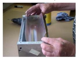
4) Put the reflector holder inside. Please press it strongly into the rounding of the reflector and fix them with M4x12 screws from the inside.
