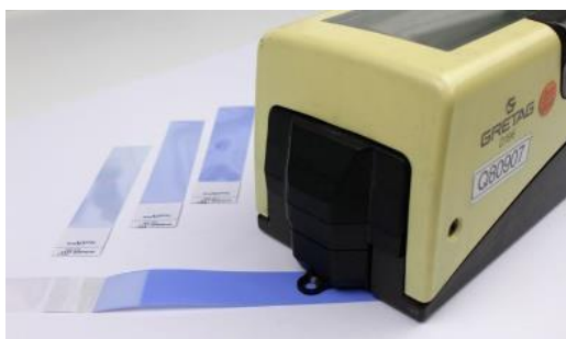
Fig. 9: Measuring the CD_B value ( B_K value, colour density black) with a densitometer
