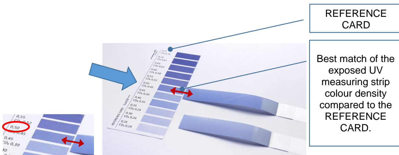
Fig. 6: Comparison of the blue discoloration on the REFERENCE CARD.
