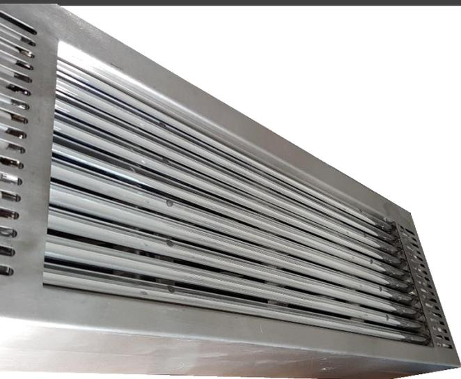
Conveyor irradiator UV-CBELT significantly reduces the risk of micro-biological contamination of the surface, packages on or around conveyor production lines.
