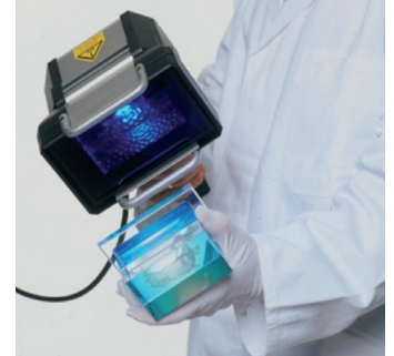
Curing of adhesives with UVAHAND 250
