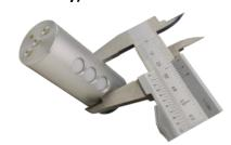
The UV Tube Integrator is UV multi-channel-measuring instrument for curing applications. It is designed to measure, record and display peak UV intensity, UV dosage and temperature\* (UV Tube 3CT) in bottle/tube machines. The sensor has to be fixed during passage in a customer-side dummy. The small size and extremely low weight of the UV Tube allows UV measurements under realistic conditions.
