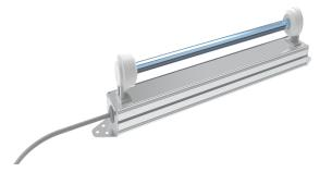
The device is a reglette built entirely in extruded anodized aluminum, IP55 protection and fitted with a reflecting screen in mirror bright aluminum, to increase the power of radiation, through the reflection of UV-C proportion that would otherwise be wasted in the opposite direction to the useful ones.
