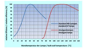
The optimum temperature of the lamp is to be considered already in the design of the UV system. For example, the cooling effect can be varied in the lamp by means of different diameters of the quartz tube. Should design changes not be enough to meet the optimal temperature, the power supply can be dimmed to meet the requirements (see also 9).
