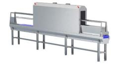
**Function:** While the employee washes and disinfects their hands, the knife basket is placed on the infeed conveyor and automatically moved through the UVC tunnel. The employee picks up the finished disinfected basket at the outlet of the system. No heat development - the sharpness of the knife edge is not affected. Optimal light isolation of the UVC lamp enables safe use for employees.
