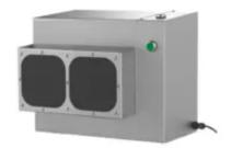
**Function:** The HD300 UV device is equipped with an actuation mechanism that starts the disinfection process by touching the trigger plates and at the same time guarantees proper and safe use. The UVC disinfection process is completed in just 5 seconds. An acoustic signal indicates improper disinfection.
