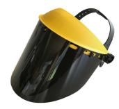
**Function:** The UV-C full face shield has a large protected view area that allows for an unrestricted field of vision when working with UV-C emitters. An adjustable snap closure allows the shield to be adjusted to the specific user. The UV-C face shield provides reliable protection against UV-C radiation in a range of 254nm. Testing: EN166
